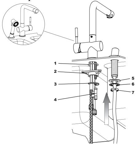
Install the fastening components to the faucet's threaded shank in the following sequence: round gasket (1), triangular flange (2), metal washer (3) and threaded nut (4) (the triangular flange can be omitted if the sink/countertop is too thick). Install the fastening items of the spray head holder in the following sequence: the flat rubber washer (5), the metal washer (6) and the threaded nut (7).
